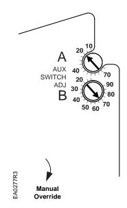
Figure 13. Dual Auxiliary Switch Dials.
